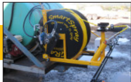
300m Hydraulic Drive SmartSpray Reel with 12m boomless jet boom to suit existing sprayer.
