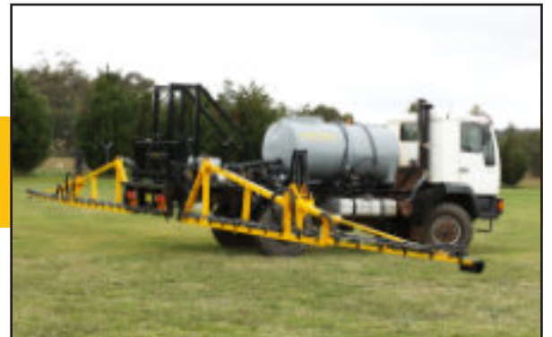
15.5m hydraulic fold and wing tilt truck mounted SmartBoom. Custom built to suit Mitsubishi Canter.
