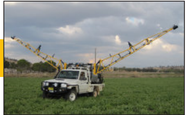
15.5m hydraulic fold and wing tilt truck mounted SmartBoom. Custom built to suit Mitsubishi Canter.
