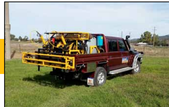
Twin Reel SmartSpray to suit dual cab tray with diesel engine, 10m SmartSpray Boom and triple nozzle boomless jet.
